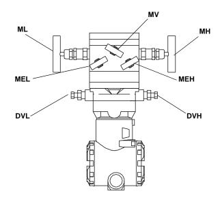
Figure 3-2. Valve Identification for Direct Mounted Models with 5-Valve Manifold
