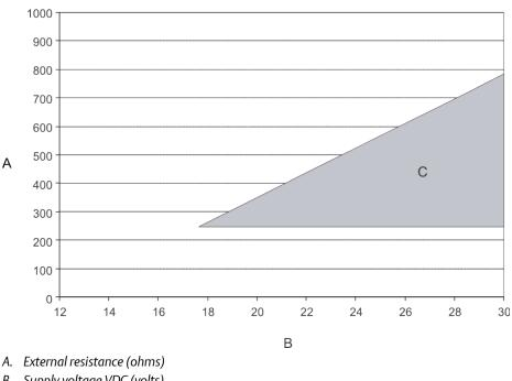
Figure C-6: Supply voltage and resistance requirements
