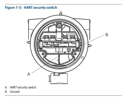
The HART security switch is the switch on the left.
