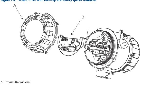
Figure 7-2: Transmitter with end-cap and safety spacer removed
