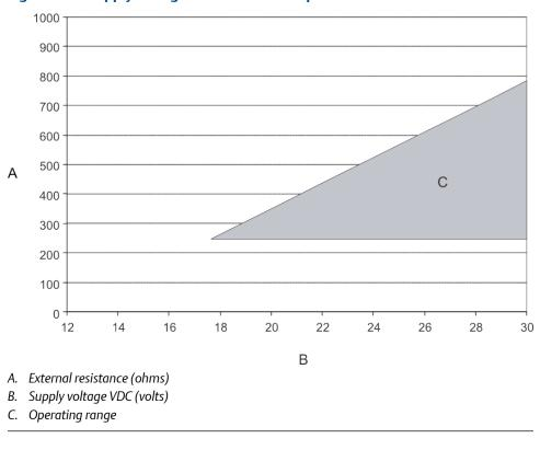
Figure C-4: Supply voltage and resistance requirements
