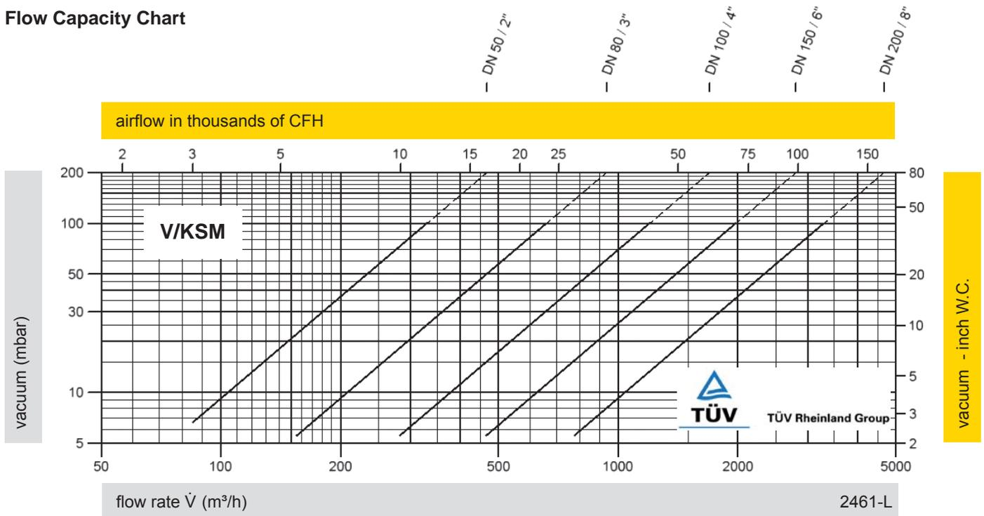
The flow capacity chart has been determined with a calibrated and TÜV certified flow capacity test rig. Volume flow  $\dot{V}$  in  $(m^3/h)$  and CFH refer to the standard reference conditions of air ISO 6358 (20°C, 1bar). Conversion to other densities and temperatures refer to Vol. 1: "Technical Fundamentals".
