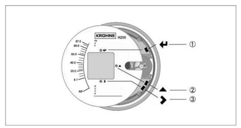
Figure 6-1: Display and operating elements
