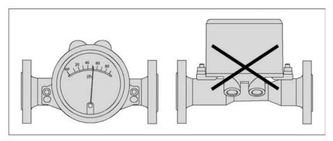
In order to comply with thermal parameters and measuring accuracy, H250H flowmeters for horizontal installation are to be installed in the pipeline so that the display is located on the side of the measuring tube. The maximum medium and ambient temperatures indicated as well as the measuring accuracy are based on lateral installation of the display.
