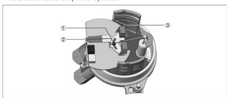
The contact module connecting terminals feature a pluggable design and can be removed in order to connect the cables.
