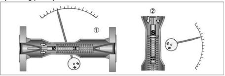
Figure 8-1: Operating principle H250H and H250U
