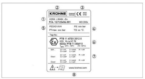
Figure 2-2: Nameplate on the indicator
