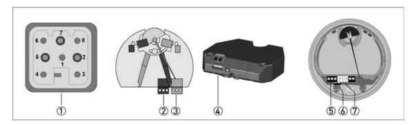
① Terminal pin assignment HAN® 7D - View of plug connection
